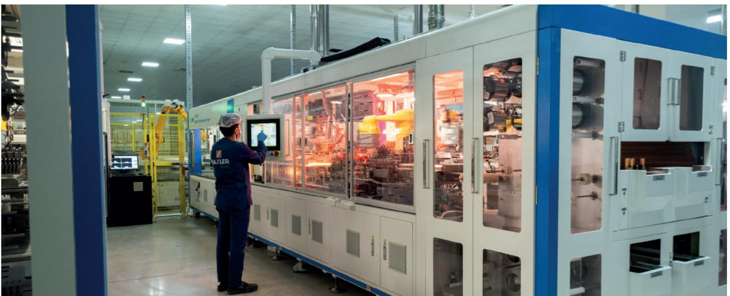
High Speed Stringer with AI+Micro Gap+Optical Inspection+EL Imagine
